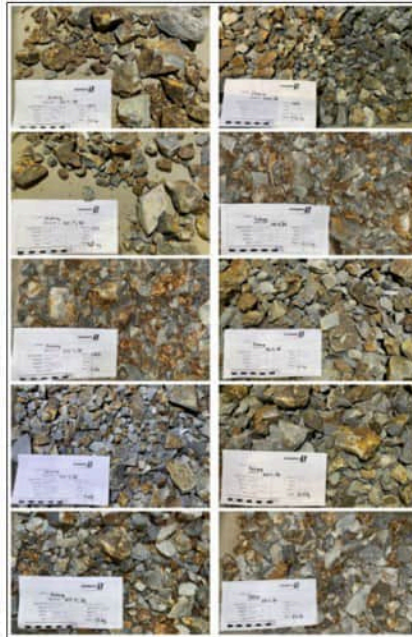
Figure 10-3: Sorter Test Products (Step 1 to 5 from top to bottom)
